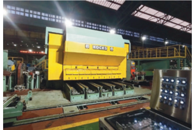
▲ Kocks RSB 370+±/5 with SCS and 4D Eagle measuring gauge
