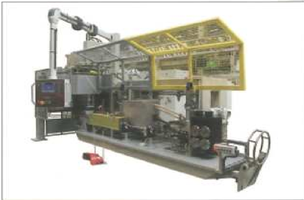
Hot drawing machines are used to reduce the diameter of difficultly transformable wire by drawing. Photo: Kieselstein
